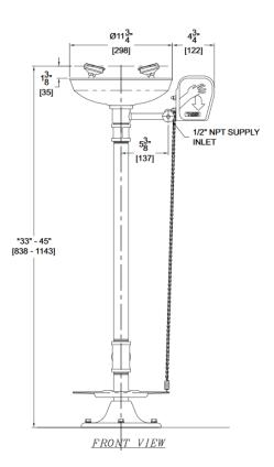
Model S0320-HFC is our free standing eye wash with foot control and plastic bowl. This unit is supplied as standard with plastic eye/face wash spray heads, an inline strainer and stay open 1/2" ball valve with a push handle. Compliant to ANSI Z358.1 standards, including safety sign and weekly testing card. Supplied with hand and foot control option giving the user a more operating flexability in an emergency situation.
